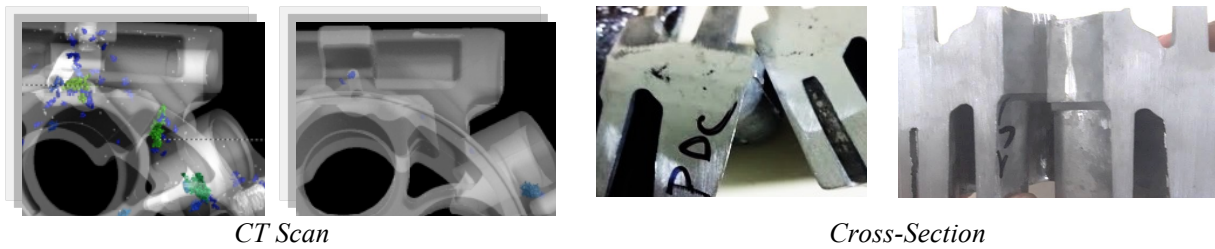
Fig. 10. CT scan and cross-section photos of HPDC (left sample) and GISS (right sample).
